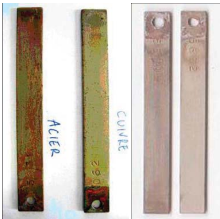
The left photograph shows \text{Ca}_3(\text{PO}_4)_2 deposits before implementation of the new monitoring and control system. After adoption, the coupons (right photograph) show no deposition. Both sets of coupons were exposed for 4 months (Fig. 6).
